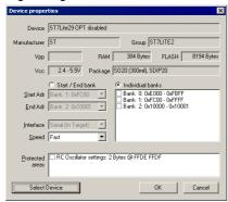
First carefully select the correct target device. A false selection may damage your target! Then select the chip area you would like to access, the sectors of the on chip-flash and the interface you would like to use. Choose one of the following options:
